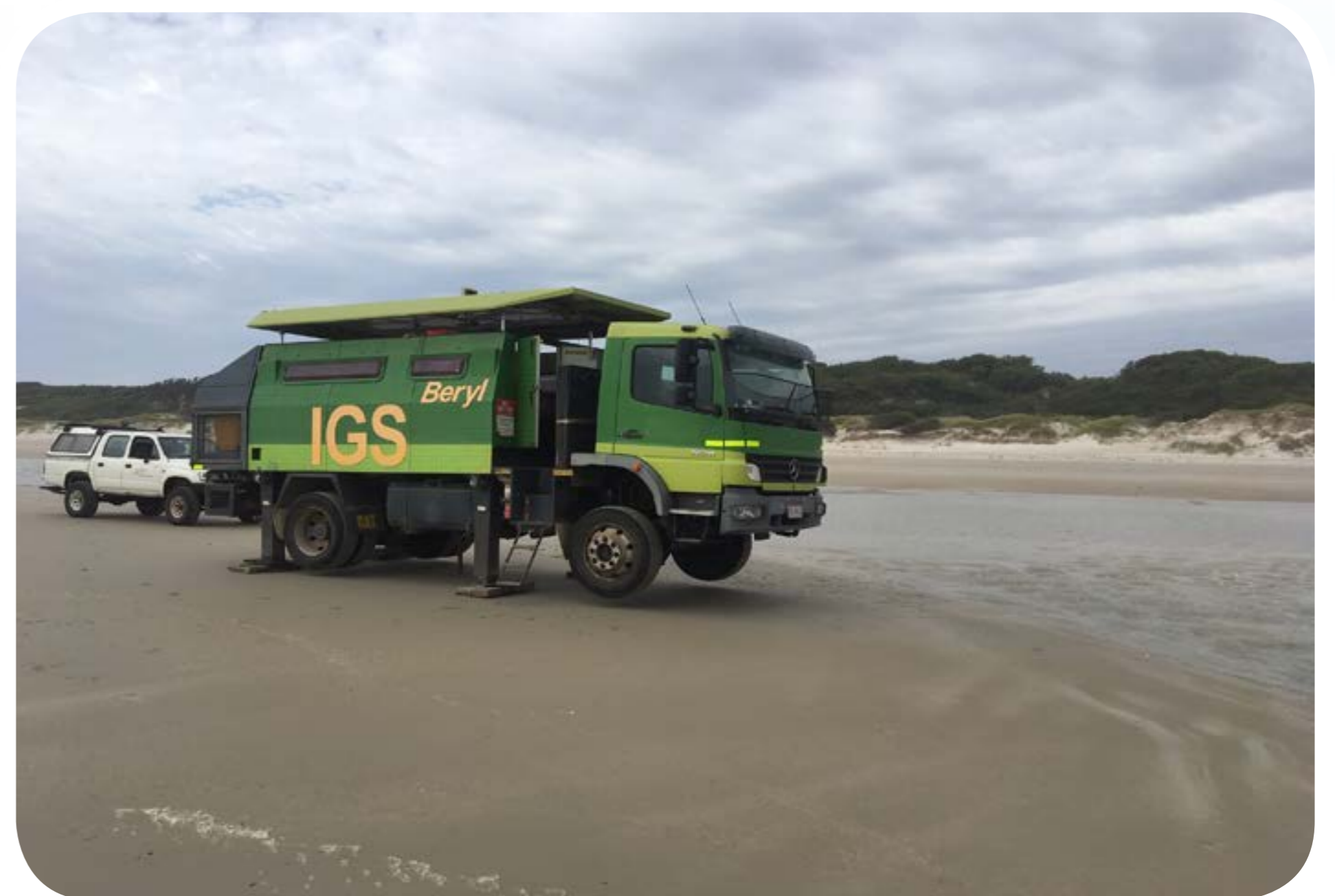
Cone penetrometer testing on Big Beach
